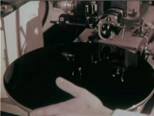
When it arrives at the studio, a guy or a gal sits there waiting for it. Back in the day (the following images are taken from a 1958 film about record manufacture for RCA Victor), audio recordings were on reel to reel tape. The Lacquer Disc (Stage 1) is set on a turntable, affixed, and then is prepared for the audio. A lathe, with a sapphire tipped cutter, etches a continuous groove into the disc once the recording starts. They constantly check to make sure the grooves are
