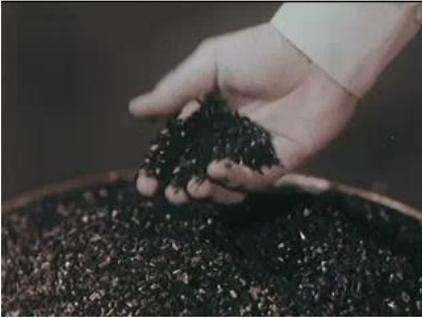
As stated earlier, Polyvinyl Chloride makes up the material that will become the LP itself. The PVC as it's commonly known is fed into the machine in granular form, where it's forced by hydraulic pressure into a soft plastic, in a quantity enough for one record.
